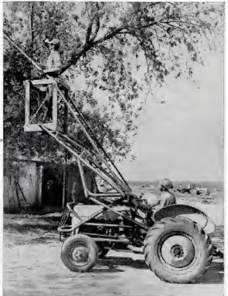
Front hydraulic lift, one of the most versatile tools on the farm, can be used as high platform, pile driver and scraper
